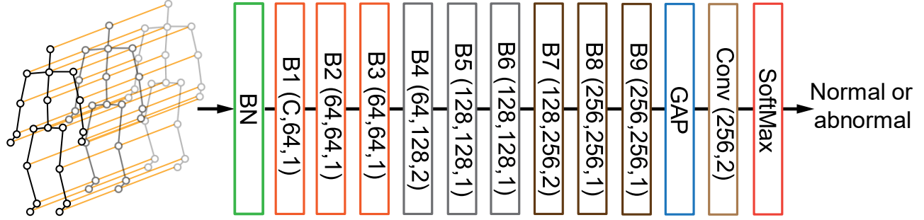
Fig. 2. Illustration of the training model. There are 9 ST-GCN blocks (B1-B9). The three numbers of each block represent the number of input channels, the number of output channels and the stride, respectively. GAP represents the global average pooling layer.
