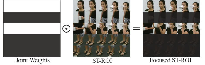
Fig. 5. Model-based fusion scheme of our MMNet. It constructs a skeleton-focused representation of the RGB modality by multiplying joint weights by the ST-ROI.
