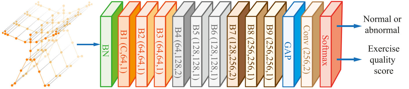
Fig. 5. Illustration of the 2T-GCN model structured with 9 GCN blocks (B1'B9). The three numbers for each block represent the number of input channels, the number of output channels, and the stride, respectively. GAP represents the global average pooling layer. The model output can then be classified by a SoftMax classifier to infer abnormality; the results will also deliver a numerical evaluation score by utilizing the probability output of the SoftMax layer.
